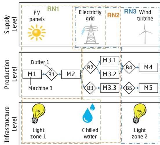
Fig. 2. Exemplary Resource Networks in a simplified production system [2].
