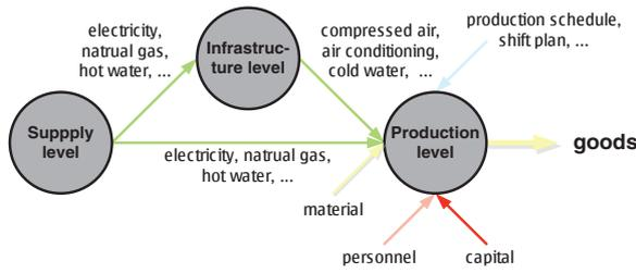
Fig. 3. Flows of production requirements in a Resource Network.
