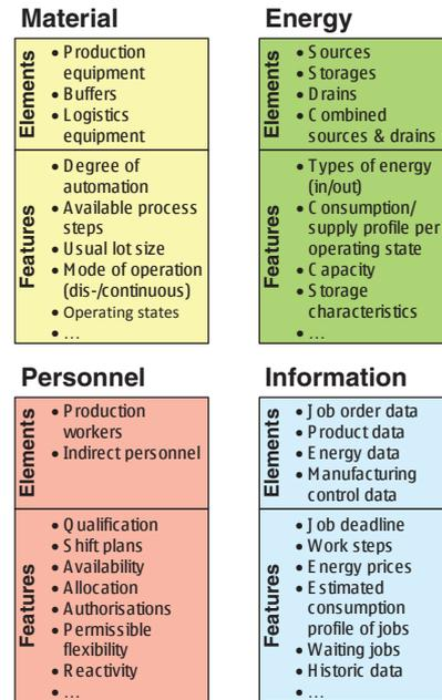
Fig. 1. Elements of the various flows in a production system [2].
