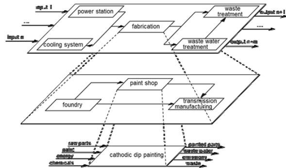
Figure 2: System structure of a component plant in the automotive industry
