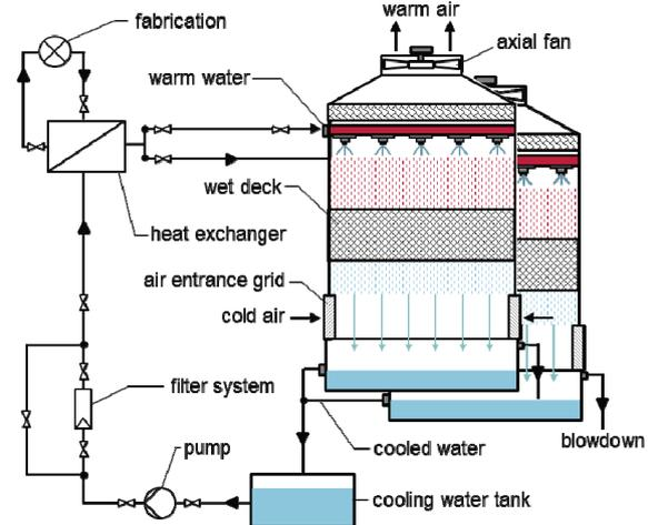
Figure 3: Cooling system
